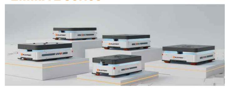
EMMA L series (Easy Mobile Mate) consists of AMRs with payload from 400kg to 2,000kg, EMMA L series AMRs also provide a lifting device without rotating plate as an option. EMMA L series AMRs can easily add various sensors or mechanisms inside or on the top for customized applications. Each AMR in this family has an optional CE complied type.
