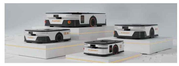
EMMA K series (Easy Mobile Mate) consists of AMRs with payload from 400kg to 1,500kg. Based on IPLUSMOBOT latest hardware platform, all EMMA K series AMRs are made by casting chassis, resulting in light mass, compact size and accurate navigation. EMMA K series AMRs also provide lifting device with or without rotating plate as an option.
