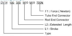
Please mention "00" in the part number if you do not require the end fittings. Some end fittings are interchangeable and must be positively secured by the customer to prevent unscrewing (i.e., loctite).
